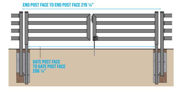
• The nominal opening between gate faces for Dual Gates is 4 ¼" when an EZ Latch is used. When not using an EZ Latch, the gap between gate faces is 3 ¼". In this case, 1" should be removed from the End Post Face to End Post Face Spacing.
