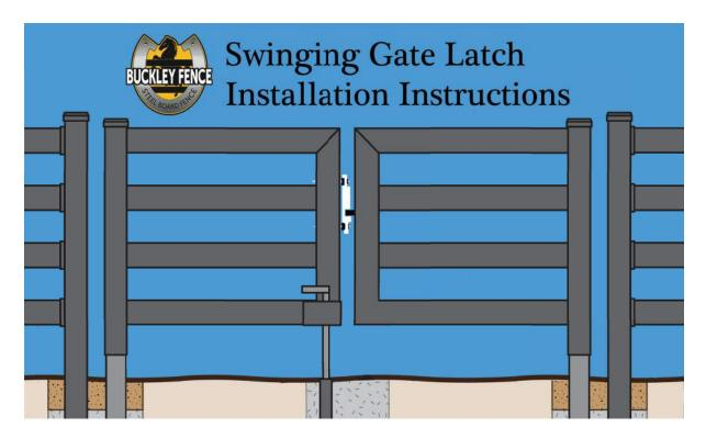
Both of the gates lower bearings can be rotated for gate level and fine adjustment of the latch and latch pin vertical positions. Adjustable Lower Bearing Video: https://youtu.be/RLkIU1px7nY Complete the gate leveling before proceeding to mount the EZ Latch.
